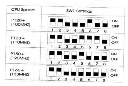
Note: SW1 PIN 1 set to "off", the Cache Mode is Toggle. SW 1 PIN 1 set to "on" the Cache Mode is Linear. CYRIX CPU uses Linear mode which is better, and the BIOS "Linear Mode SRAM Support" must enabled.
